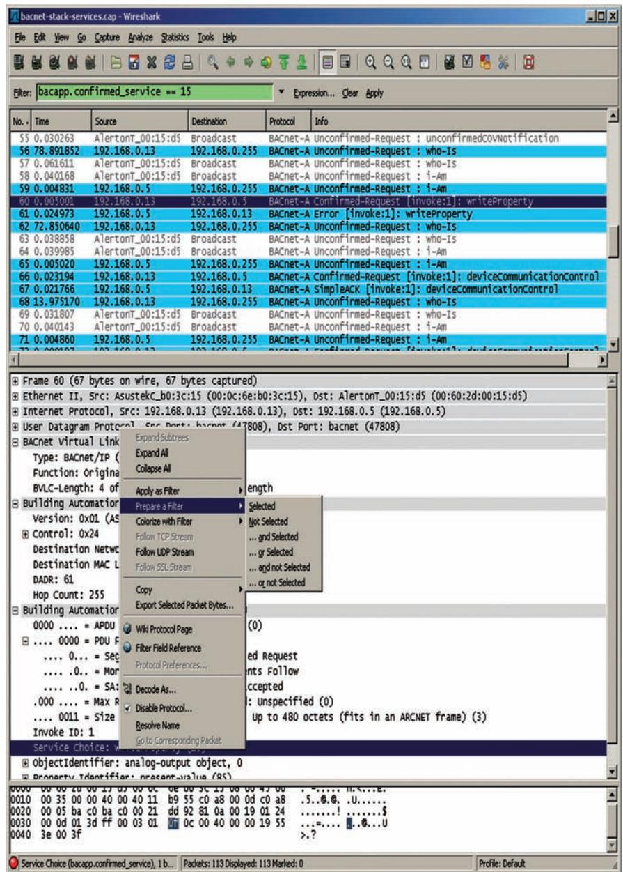
Figure 4: Wireshark default display, showing the ability to prepare or apply a display filter.
