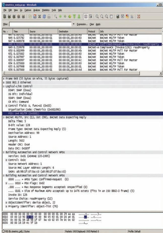
Figure 2: Wireshark and a BACnet MS/TP capture from an external interface, which sends Ethernet SNAP protocol packets.
