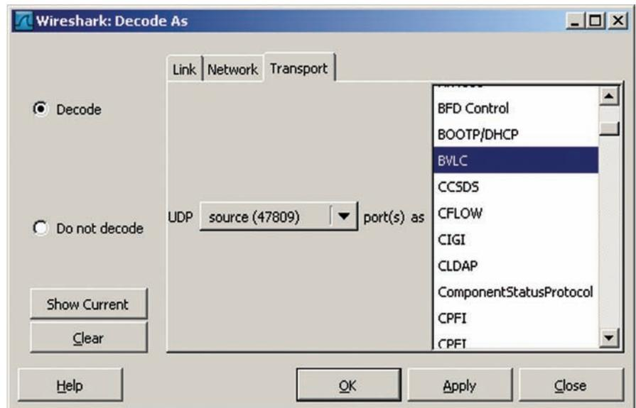
*Figure 5: Wireshark “Decode As” dialog showing BACnet/IP port 47809 decoded as BVLIC.*
