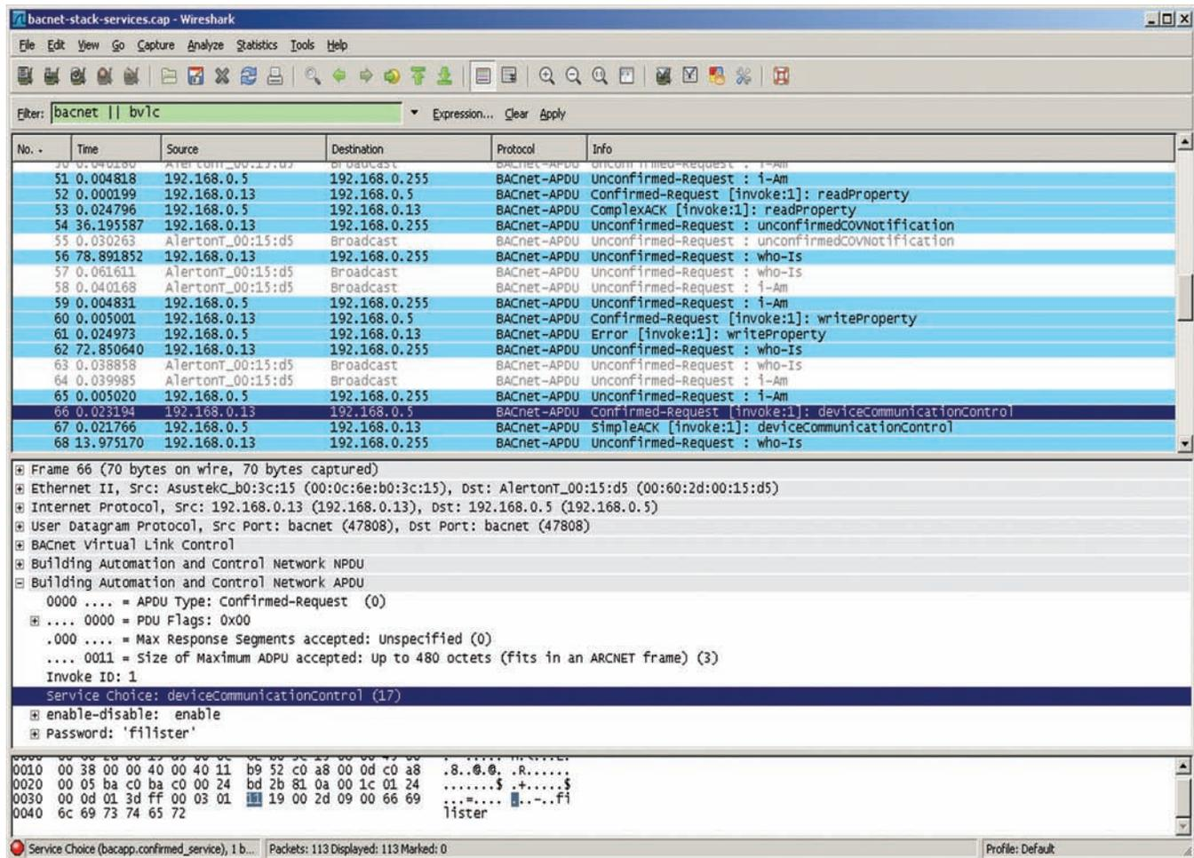
Figure 1: Wireshark displays a variety of BACnet services from various sources, and is useful for troubleshooting, developing, or learning about the BACnet protocol.
