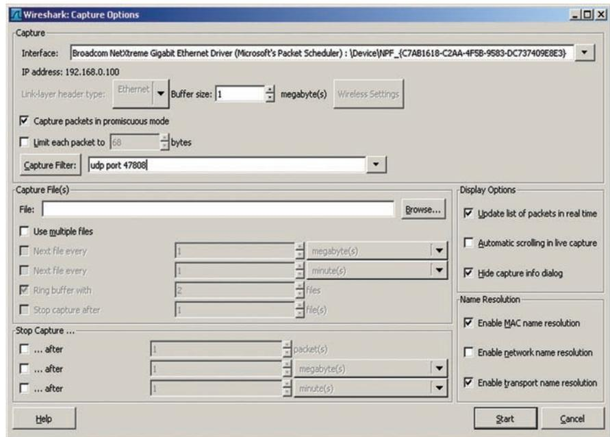
Figure 3: Wireshark Capture Options dialog box allows control of the capture display, name resolution, capture files, capture interface, capture filter, and the ability to stop after so many packets, bytes, or time.
